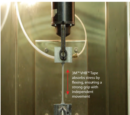
3M™ VHB™ Tape GPH-160 allows stiffeners to be bonded prior to a paint bake cycle.
