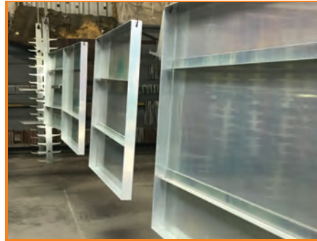
3M™ VHB™ Tape GPH-160 allows stiffeners to be bonded prior to a paint bake cycle.
