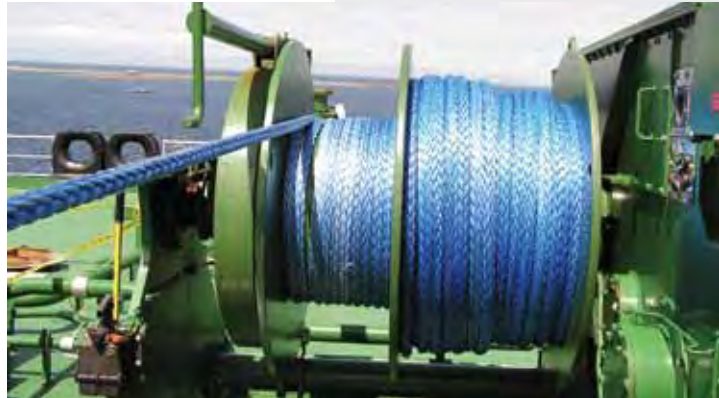
Eight to ten wraps must always remain on the tension side of the split-drum winch at the line's full extension.
