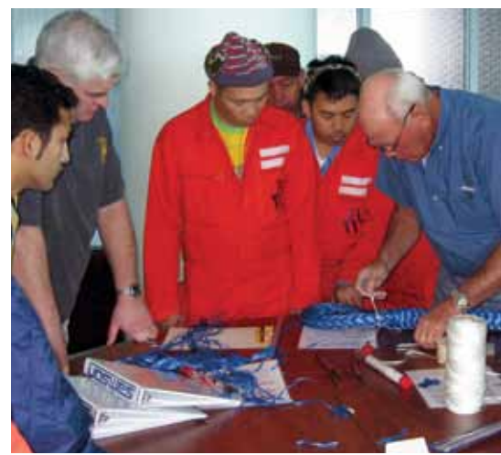
Samson field support technicians frequently assist with wire rope mooring line replacements while vessels are underway, complete with crew training in splicing, inspection, maintenance and proper rope-handling techniques.
